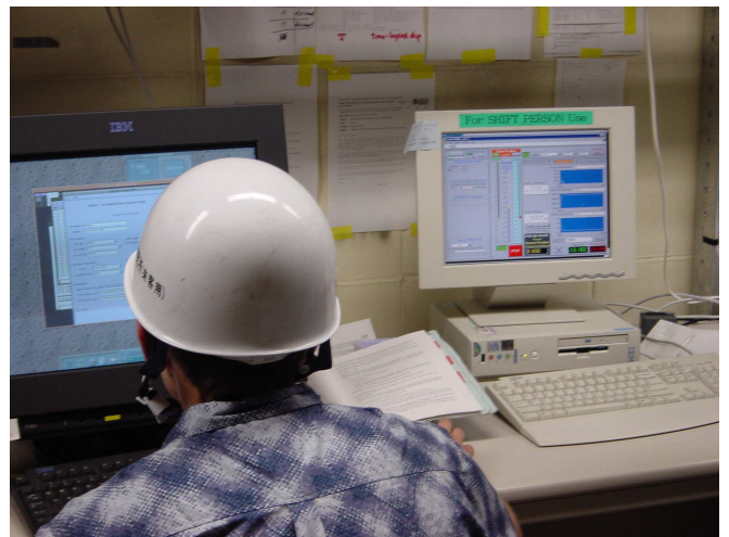
FIG. 1: A KamLAND shift operator controls the data acquisition system during a calibration source deployment. The computer on the right controls the position of the calibration source inside of KamLAND.
