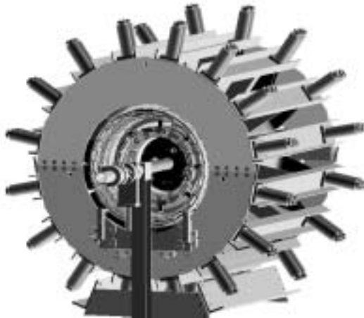
Figure 2: MuCap detector showing scintillator barrel, cylindrical wire chambers and vacuum pipe supporting the hydrogen vessel.
